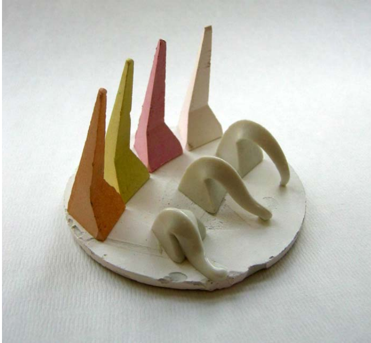
Picture 3. Orton cones are designed to indicate a temperature interval. They are usually used in sets of three which reacts slightly different to the temperature, and can thus indicate which temperature was actually reached during the firing. The cones in the right row that accompanied the mugs during the firing shows that the temperature interval for which they were chosen was complied with. At too low a temperature the cones would not bend enough and at too high a temperature they would bend too much. The left row show unused cones for different temperatures.
